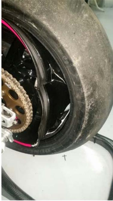
Front and rear tyres were inspected and were in good condition with the front tyre still inflated. The data showed the rear tyre pressure was at the recommended pressure of 1.4bar at the time of the incident. This confirms that the rear rim failure is a consequence of, and not a cause, of the accident.
